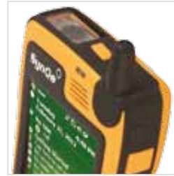
gSTAR-6200 with antenna and Scanner (Barcodes & RFID tags)
